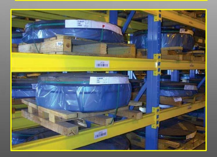
Acrow's Extra Heavy Duty Frames, which use heavier upright sections, have a capacity of 30 tons or more. In addition, Acrow has the ability to custom-create heavy-duty racking for any requirement.
