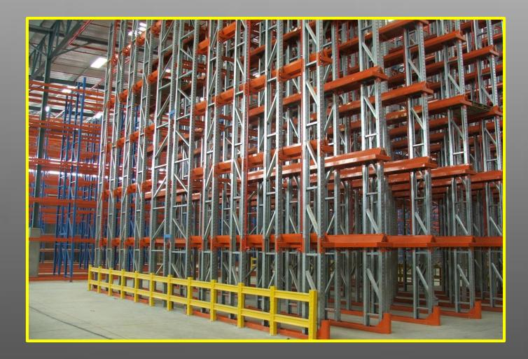
The Drive-in system is used to ensure maximum usage of floor area when the warehouse space is minimal. This system is often used in the cold room environment saving energy and warehousing costs.
